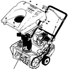
Lubricate chute control flange. Coat flange with a clinging type grease such as Lubriplate.
